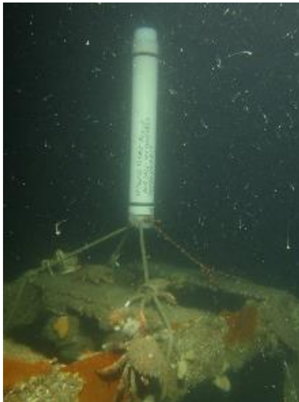
Figure 6.10.5. Static acoustic data logger attached to seabed frame located at OMS site.
