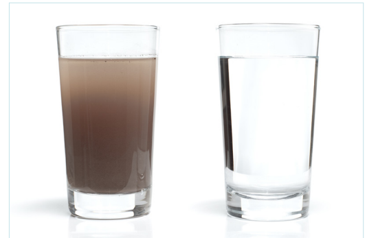
On the left a glass of water with a high turbidity level. On the right a glass of water with a low turbidity level.
